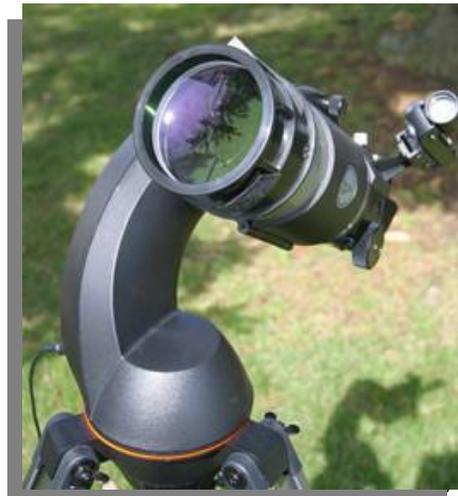
false color to tolerable levels, the focal ratio must be around three times the size of the objective in inches, for an 80mm (3.15 inch) scope, this means that the focal ratio should be around f9. The NexStar 80 is an f5. As you might expect, false color abounds. Even at low powers, bright objects like Sirius, Luna and Venus are ringed with a purple halo.
