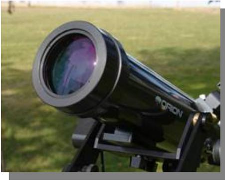
In long duration testing, I've discovered that on one of the two samples I've been using the lens cell has worked itself loose and needed to be tightened. Obviously this is not something that you really want to see.
