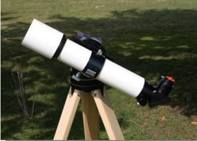
supplied tube ring, while functional, is not the quality I would expect with a premium refractor in this price range. I was unable to mount it directly to a Gibraltar, Telepod Head or a G11 universal plate, and wound up securing the OTA with a single screw. While this worked, I wouldn't recommend it for constant use.
