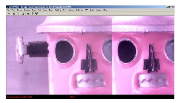
This snap was taken in full auto mode, with automatic white balancing. Note that the colors are washed out – this is because there is no IR blocking filter built in and IR is leaking into all R, G, and B channels, effectively mixing white into the picture and reducing saturation. Adding an IR block filter – not included - gives the correctly saturated image (also taken in full auto mode):
