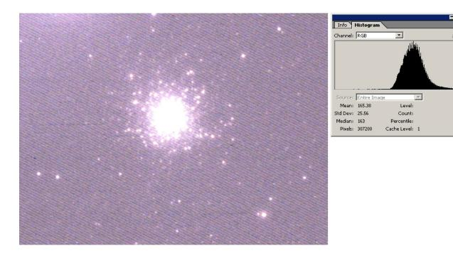
There's a little bit of electrical noise (the diagonal banding) that I'm not sure is intrinsic to the SAC7, or part of my setup. I took 4 images and stacked them (averaged) to reduce the effect and reset the black point to eliminate the dark current image offset:
