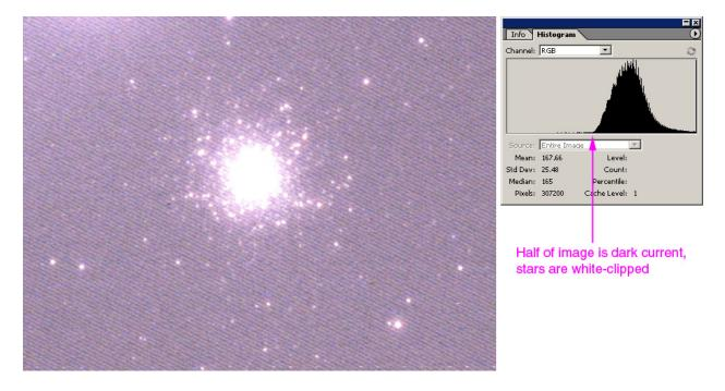
At 60 seconds, about half the image dynamic range is taken up by dark current (ambient temperature was in the mid 60s, a cold winter night would dramatically reduce dark current), and the stars are clipped, but the skyglow histogram is intact, so this is the longest reasonable exposure to take under these conditions.
