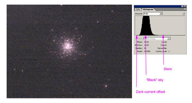
The histogram is now displaced to the right, showing some accumulation of dark current. At 15 seconds, about 10% of available signal dynamic range has been used up by the dark current, so we can definitely increase exposure some more.
