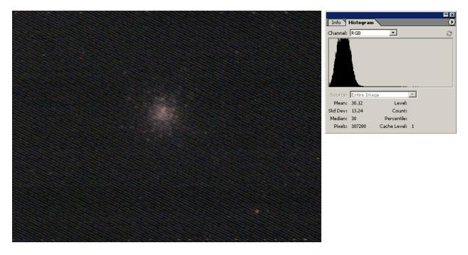
At 5 seconds exposure, the histogram is pressed to the left, indicating that very little dark current has accumulated.
