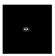
It will be noted here that a scope with central obstruction of 20% the diameter of the full aperture, even though it will reduce the light in the visible disk and put more light into the first diffraction ring, will have
