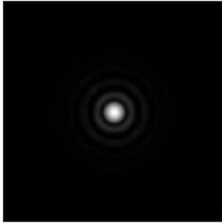
**Spherical Aberration** - this occurs when the rays parallel to the optical axis do not come to focus at the same point. Typically in the case of a lens or a spherical mirror the outer rays intersect closer to the lens or mirror than the inner rays. There is no one common focus, but rather a region where it's all equally bad. This is called the zone of confusion as there is no one true exact focus point. Do not confuse the zone of confusion with the depth of field found on longer
