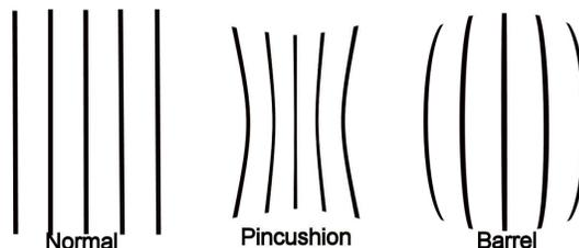
**Negative or Barrel distortion** - the slats on the will bend inward
