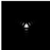
Pinched optics can also cause an aberration in a similar class as astigmatism. If a lens or mirror is too tight in its cell, the optic may get pinched enough to effect the optical figure. If that's the case, the pinched optics can be spotted as triangular or trapezoidal stars. Alleviation of this may involve loosening the optic in it's cell, designing a new support system or simply letting the optic come to ambient temperatures.
