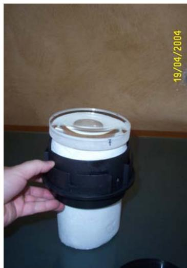
Ok, now it's time to put some marks on the edges of the lens elements, as shown below.
