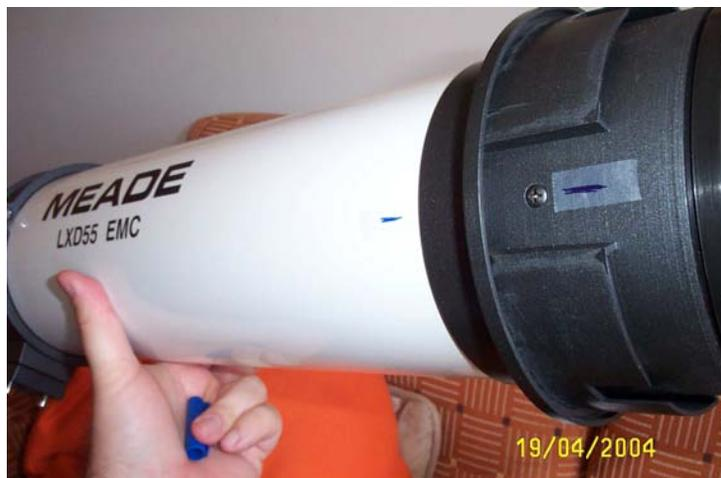
This is an important step because it will allow you reassembling the cell back on the tube without rotating it, assuring that you'll preserve the collimation set by the manufacturer.
