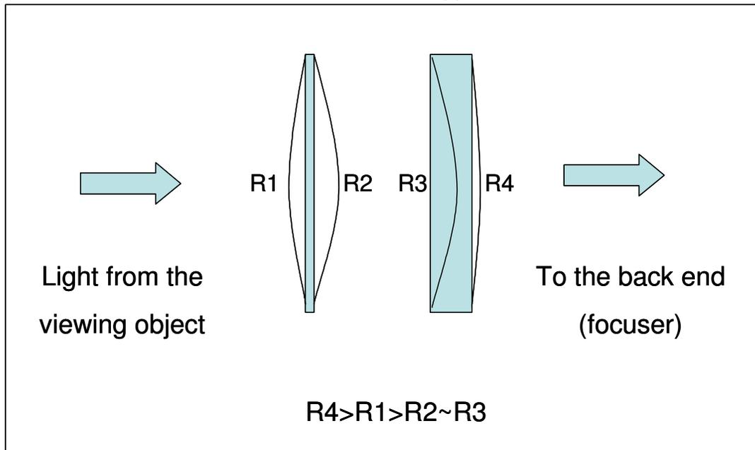
The scheme above is all that you must keep in mind when reassembling the lens in the AR5's cell in order to avoid any element misplacing or flipping.
