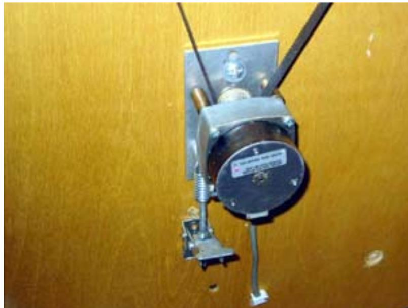
A spring clutch is provided which permits relaxing the belt so manual motion is possible. Again, this won't affect DSCs but will cause Roboscope to lose position information. Supplied rollers are used to replace one or more of the usual Teflon pads to permit the elevation motion to be more free. Due to the weight of my system and the small elevation bearings I replaced all the Teflon pads with rollers on this one. To remove the mirror box, it is necessary to first release the spring
