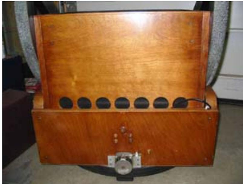
Tech2000 also offers a rim drive for azimuth, which drives on the outer diameter of a round ground board. I considered this for the Starsplitter since it has a circular ground board, but had no easy way to face the perimeter into a perfect circle. The azimuth rim drive also includes an adjustable slip clutch which makes it unnecessary to disengage the drive for manual motion of the telescope; this clutch looks similar to that used in the declination tangent drive add ons for the Meade LX series.
