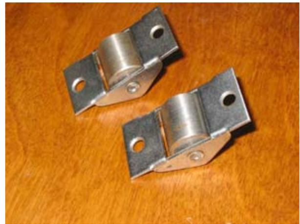
These are installed a little less than 120 degrees apart, either side of the center front of the rocker box bottom. Then the motor is mounted to the rocker box rear center so that a knurled wheel (about 2" diameter, 2" width) drives against the top of the ground board to rotate the rocker box. This requires notching out the bottom and back panel of the rocker box.
