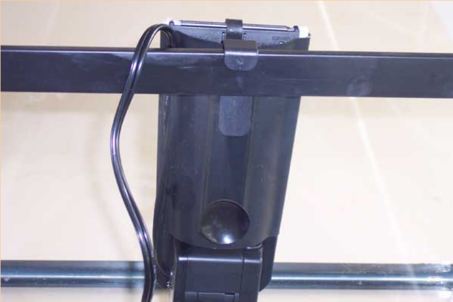
Tank clip (top), bottom suction cup. A 2nd suction cup can replace the tank clip
