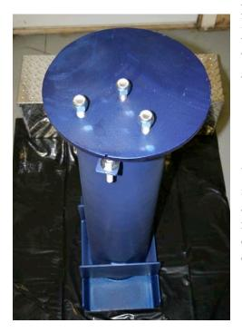
your installation setup. When the pier is installed, I remove the cap and place a plastic bag down in the pier tube. I then fill the plastic bag with "play" sand. This gives about 80 bounds of additional dampening stability.
