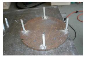
Notice in the picture there are three holes drilled near the center of the cap plate. These three holes will attach the bolts used to secure the mount base plate. I drill 5/8s inch
