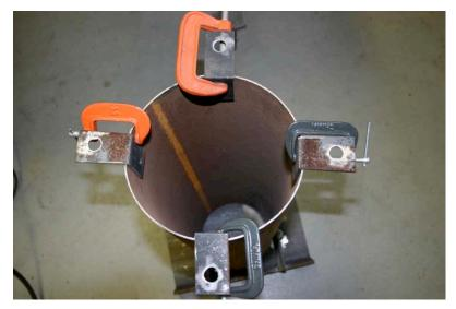
Take four pieces of 2 inch angle iron and drill a 5/8 inch hole in one side in the center. You will use
