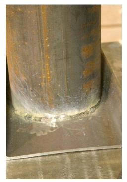
Before I started welding the side plates on I "touched up" the welds around the base with the grinder. It was easier then.
