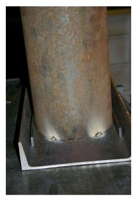
down the main tube to the base plate in four places opposite each other. Center the tube in the base with the "U" facing up. Notice the metal bars placed beside the tube to center it in the channel.
