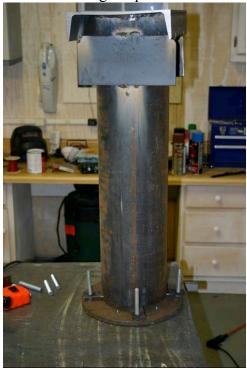
Carefully slip the tip of your wire welder under the edge of the flange and tack the bolts
