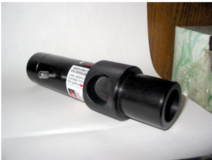
Here the switch and the side window can be seen
