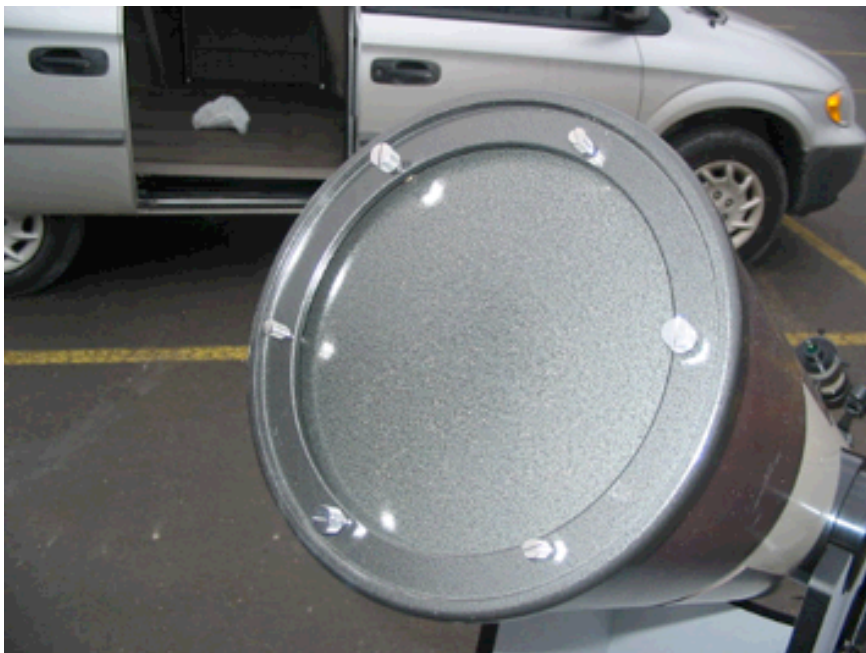
Here are the primary mirror's collimation screws. Note the warning below about placing the telescope in this position!
