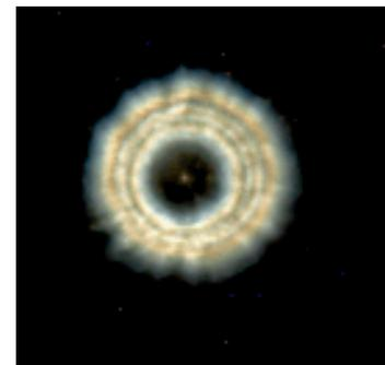
...and with the secondary shifted .3mm (according to the handbox) outside of focus:
