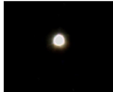
And here it is with the secondary shifted .3mm (according to the handbox) inside of focus:
