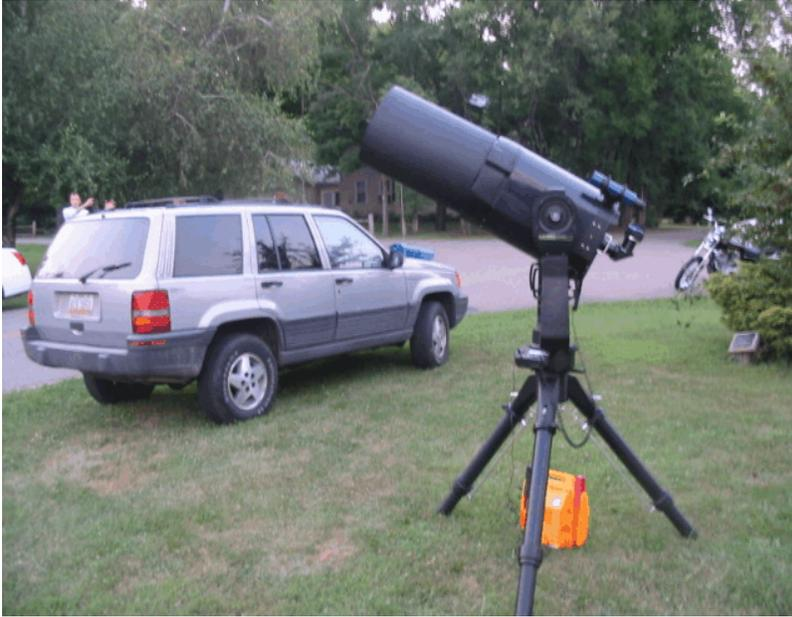
out to the field. As can be seen in the photo, I continued to ignore the battery holders in the telescope, using instead my trusty jumpstart battery pack from Harbour Freight and a DC cable from Scopestuff. The tripod was easy to transport in four pieces and went together very easily at the site. Leveling the tripod was very quick using the provided clutch release
