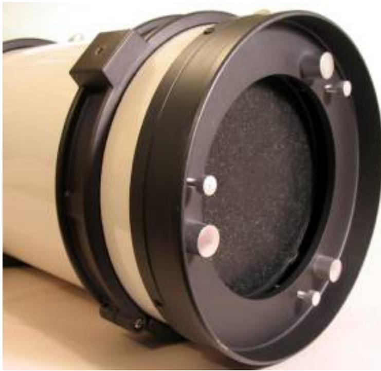
**Figure 6.** Rear view of the scope showing the three collimation screws and corresponding locks.
