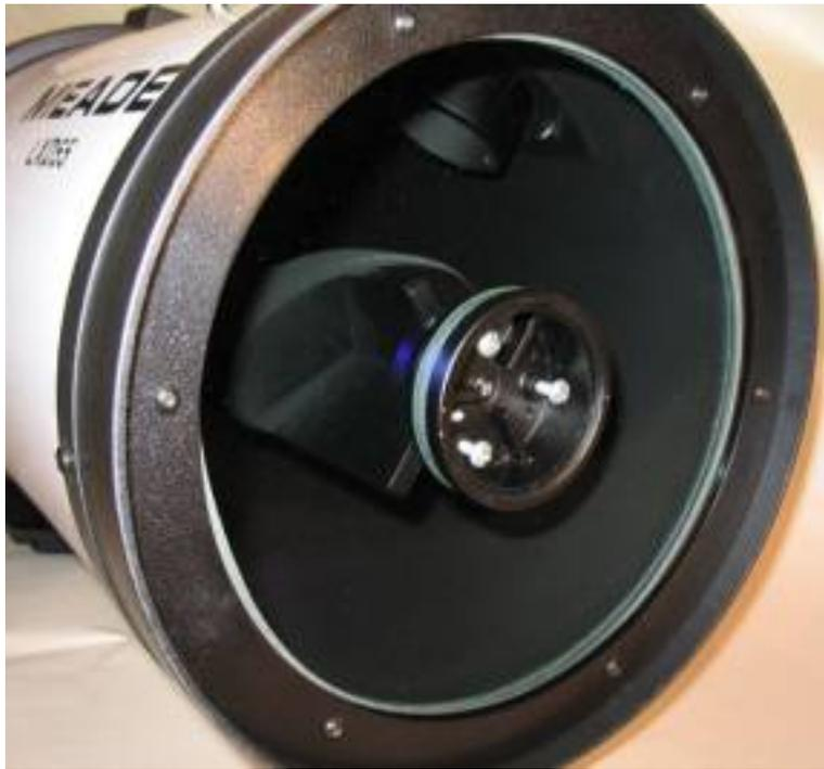
**Figure 7.** Visible here is the very large secondary mirror and its collimation screws. Note that part of the aperture is blocked by a misshapen paper gasket.
