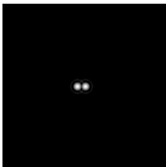
An obstructed scope, depending on the area of the obstruction, may put two or three times as much light into the first diffraction ring while reducing the amount of light in the visible disk resulting in a slightly smaller visible disk.
