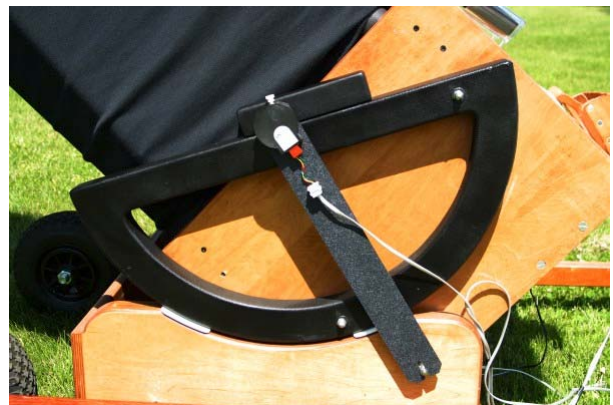
ALT encoder installation on 15" Truss
