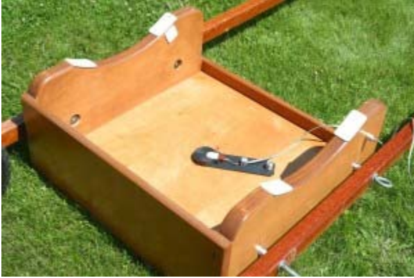
AZ encoder installation on 15" truss
