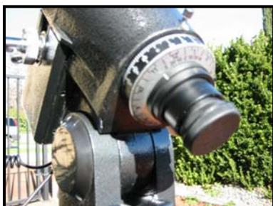
As with other CG-5 clones, the EQ-10 has a nice system for adjusting latitude and azimuth for good polar alignment. The polar alignment scope has a reticle that allows alignment in both hemispheres. Curiously, the focus of the polar scope appears relatively fixed – for persons with 20/20 vision. Take off your glasses, and it’s hard to adjust the focus enough to sharpen the images.
