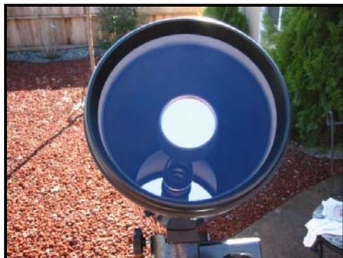
A plastic dustcover for the corrector end of the OTA is furnished. The cover has an off-center 1-5/8" diameter opening that is covered with another plastic cover. I'm not certain what the purpose of this is, other than to provide an unobstructed small aperture viewing option. The dust cover fits tightly, and I have learned to remove the cover from the smaller opening to make removal and attachment of the dust cover easier.
