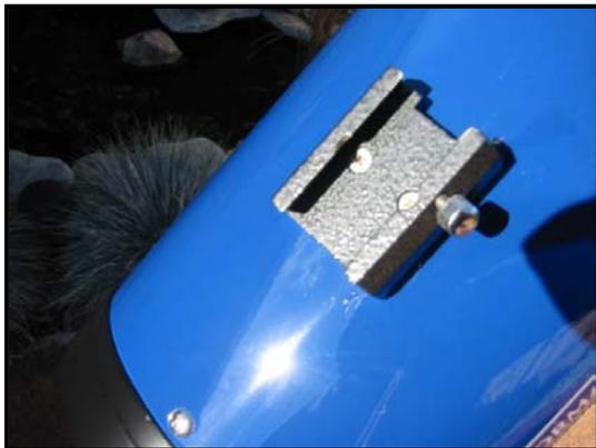
One problem I experienced was the mounting of the finder dovetail. It was not in line with the optical axis, and resulted in making it impossible to align the finder. This problem has been reported by at least two other owners. I found that by loosening the two mounting screws, turning the dovetail slightly, then retightening the screws solved the problem.
