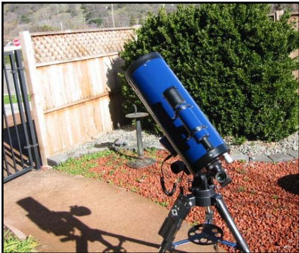
The mount itself is reasonably stable. At higher magnifications (186x), a sharp rap on the OTA or tripod would cause vibrations to last no more than 2-3 seconds. The use of vibration suppression pads reduced this to 1-2 seconds. The included setting circles are useable, and they allow you to place an object within the finder's field of view.
