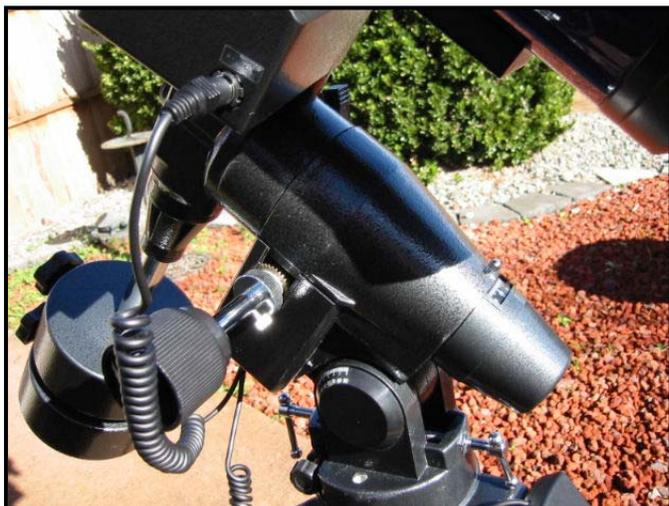
Depending on the ambient temperature, the mount is very stiff when rotating on either axis. At room temperature, it isn't too bad, and if you close your eyes, you can pretend that you are moving a huge observatory telescope on a precision engineered mounting. The stiffness makes the OTA feel smooth and massive. When the temperature gets below 40 degrees, however, things start to get difficult. You have to use two hands to turn each axis. This stiffness is well documented on sites like
