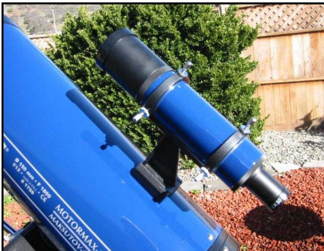
Alignment of the finder isn't too difficult once the dovetail problem is corrected. I do dislike the two-ring, 6 alignment screw setup, however, as it takes a bit of fiddling to get things just right. The alignment screws are metal – to minimize damage to the paint on the finder's OTA, plastic strips are provided that fit between the screws and the OTA.
