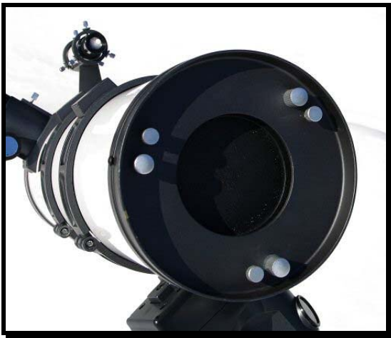
Primary collimation and lock screws
