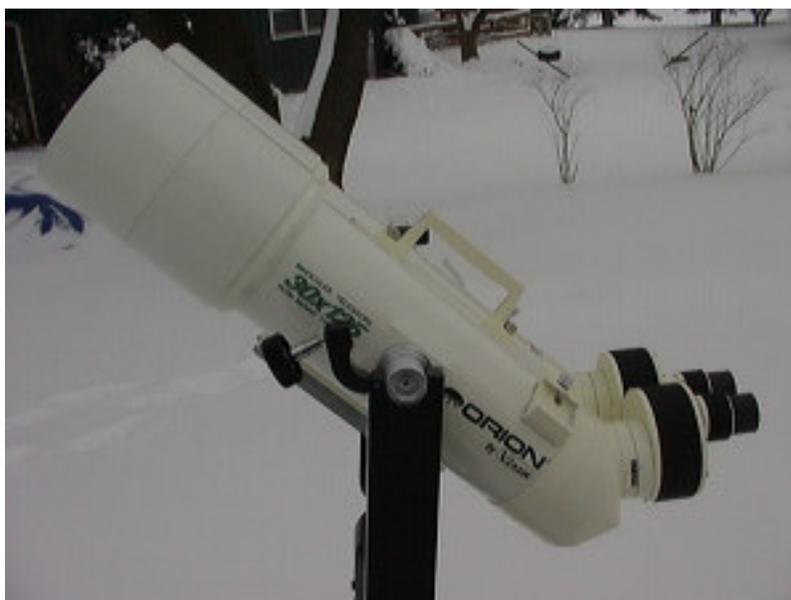
Permanently attached to each side of the binoculars are small circular knobs encased in teflon. The knobs are attached at the balance point of the binoculars, which allows the binoculars to be moved in the up-down direction without requiring any counterweights. The binoculars then attach to the fork arms by sliding these 2 teflon coated knobs into the clamshell assembly at the top of each fork arm. A single
