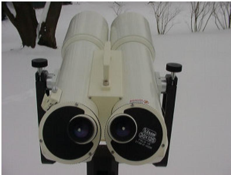
The eyepieces have full interpupillary adjustment. The entire turret that each eyepiece sits in moves in a circular manner allowing the user to adjust the distance between the eyepieces to fit their comfort zone. Each turret has a texturized rubber ring running along the outside that gives the user a gripping surface when adjusting the interpupillary distance.
