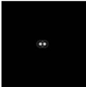
It will be noted here that a scope with central obstruction of 20% the diameter of the full aperture, even though it will reduce the light in the visible disk and put more light into the first diffraction ring, will have almost no discernable affect on the overall resolution as compared to an unobstructed aperture of the same diameter.
