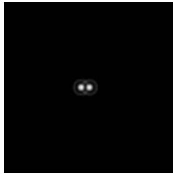
If the stars with separation at the Rayleigh limit of 1.6" were faint and had a visible disk just a hair less than 50% the diameter of the Airy disk, you would be able to see a thin line of separation.
