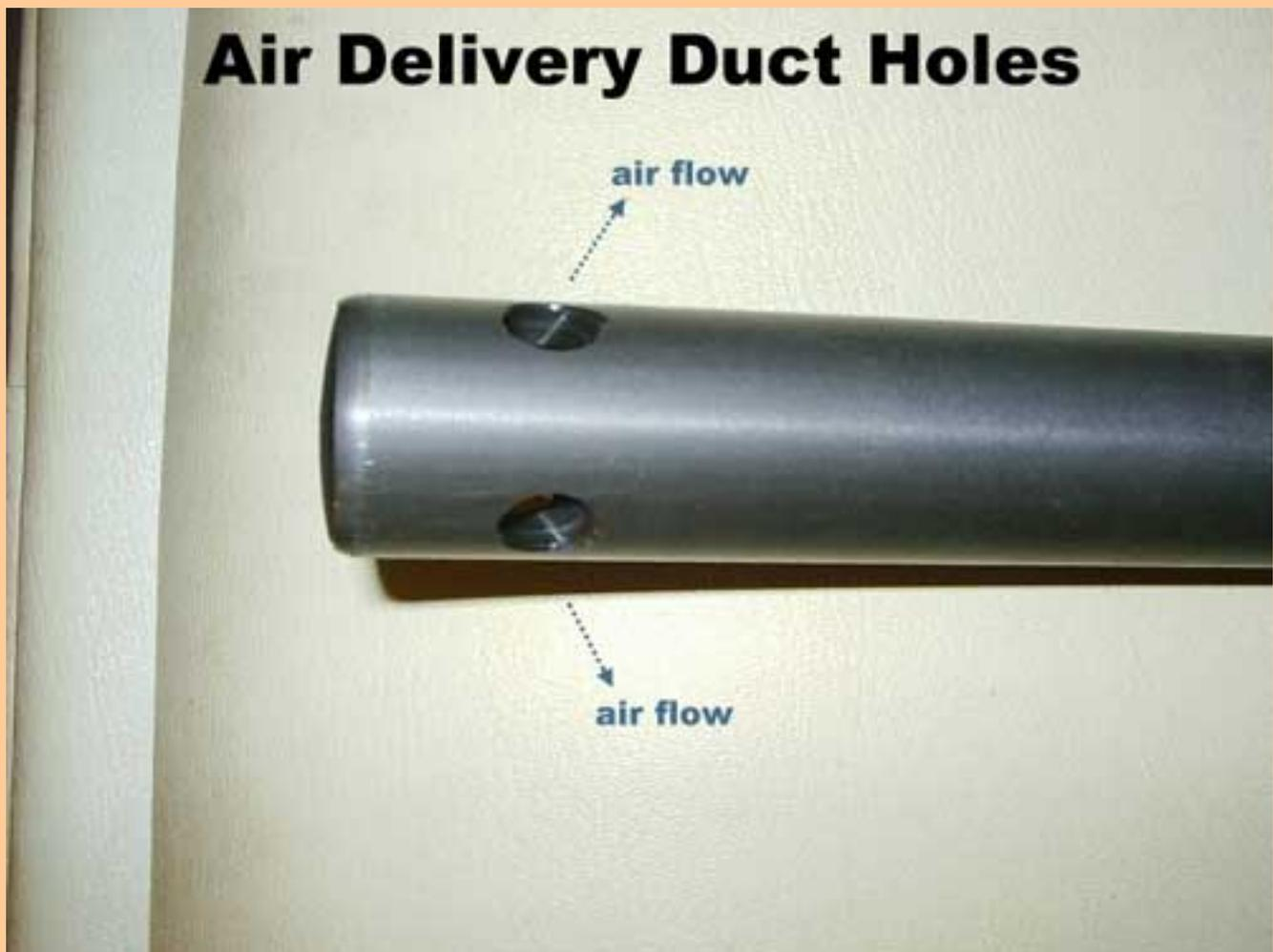
At the far end of the Air Delivery Duct are four small angled holes in the *\*sides\** of the tube which allow air to flow radially outward from the tube and slightly backward to prevent any air from directly
