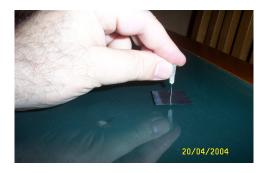
Check the holes diameters, using the slide projector method suggested by Suiter (\*) and choose 2 of them that have diameters under 0.3mm. I chose one of 0.19mm (to be my "Artificial Antares") and another one of 0.28 mm (to be my "Artificial Arcturus").
