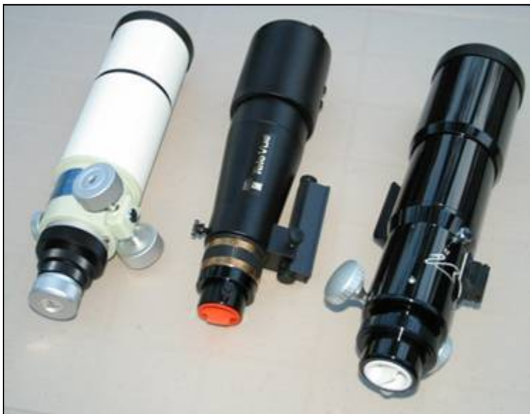
Tak FS-60c, TV 60, WO 66 Petzval Note the TV dew shield is extended, the Tak's is fixed, but it requires an extension tube to reach focus, and the 66 Petzval's dew shield is retracted
