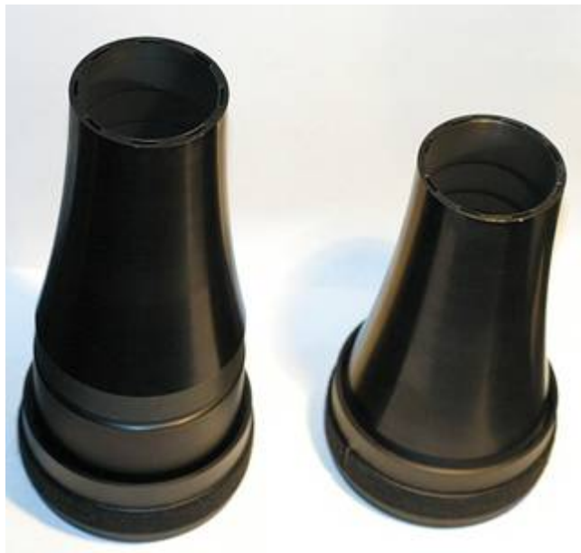
The ZenithStar 80's baffle system also serves as a lens retaining ring, and was the cause of the vignetting. On the left, the "fixed" baffle (note the extension tube), on the right, the older one that created the vignetting problem – both are shown attached to the lens cell.
